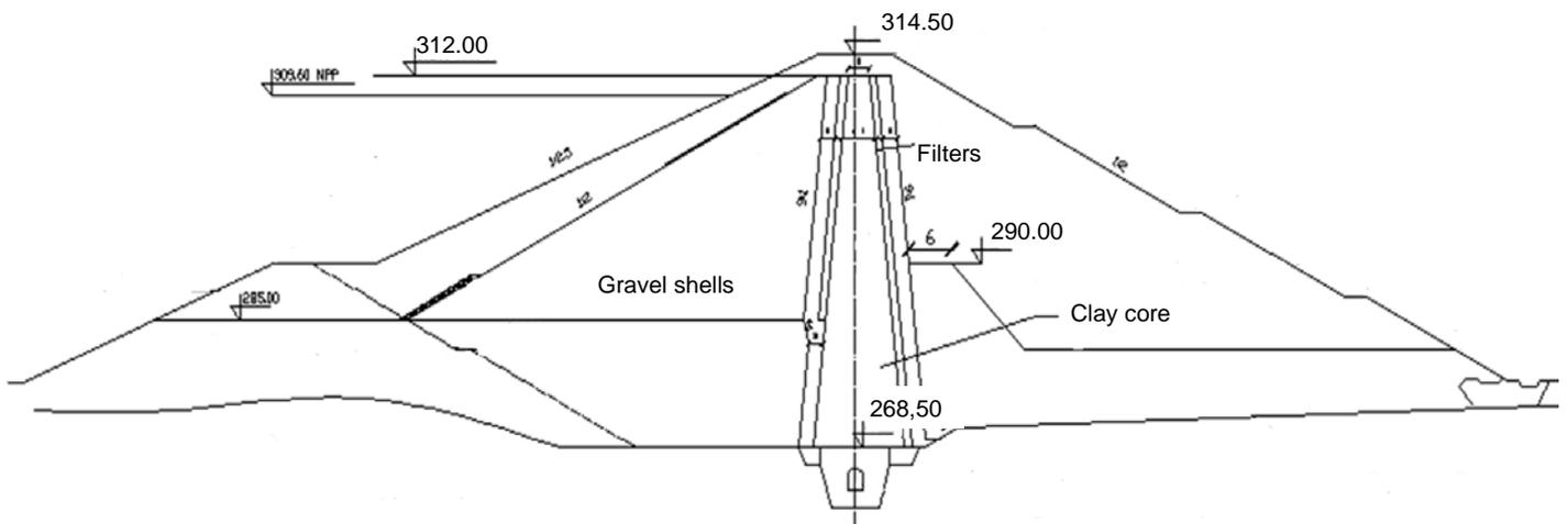
Fig. 2. Typical cross-section of Świnna Poręba Dam.
