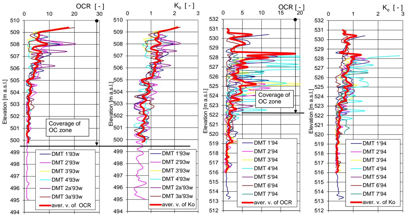
Fig. 7. Example of DMT results (performed during construction of Czorsztyn Dam in the years of 1993 and 1994).
