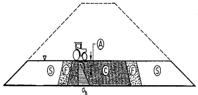
Fig. 6 State of the stress in the core of dam during the compaction process: A – increased horizontal stresses as a result of compaction, C – core, F – filters, S – shells.
