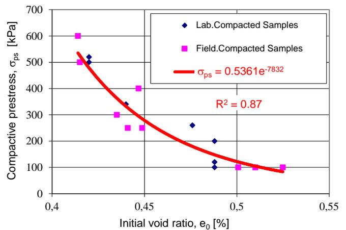
Fig. 12. Relationship between compactive prestress  $\sigma_{ps}'$  and initial void ratio from oedometr tests of laboratory and field compacted soil samples (Skutnik, 2002)
