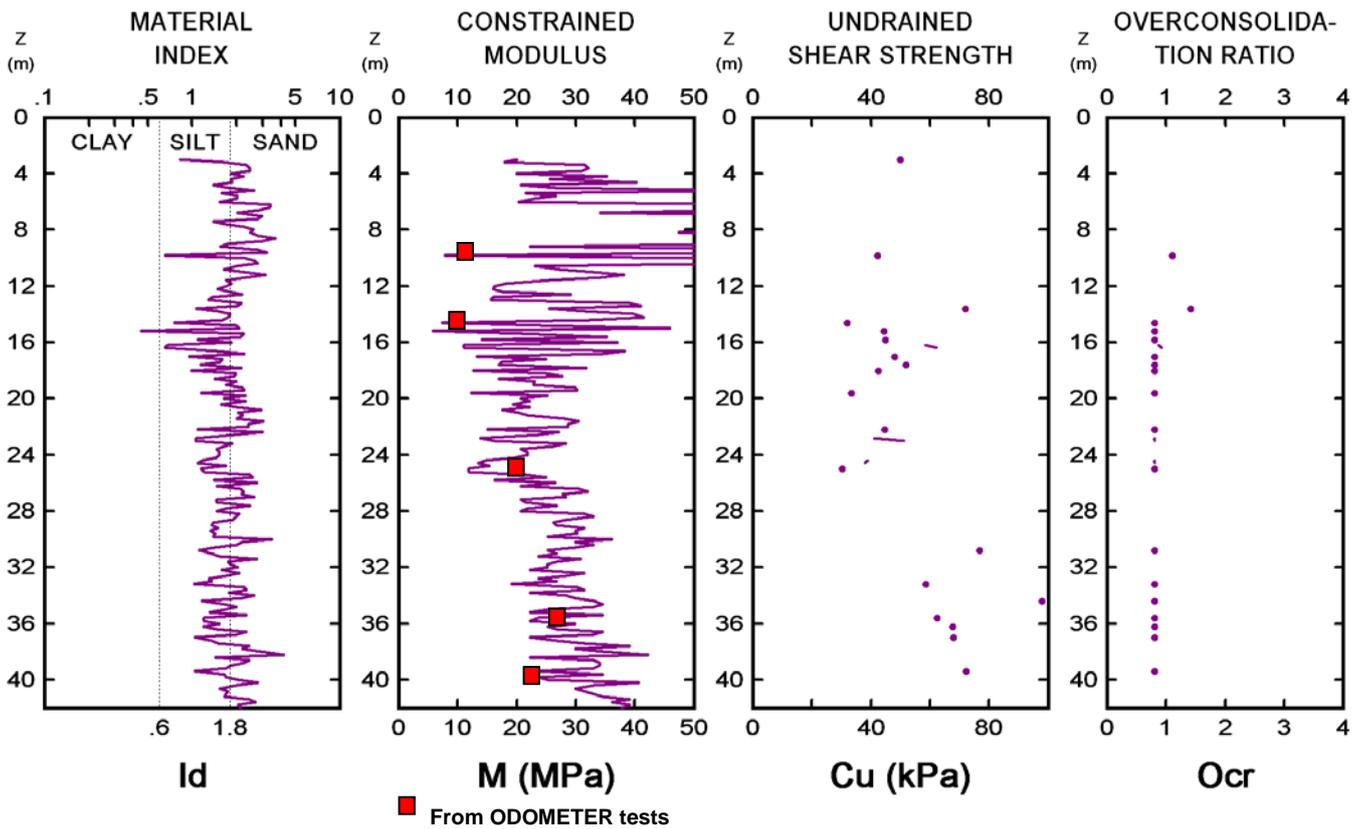
Fig. 5. Example of DMT result (performed two years after completion of the dam core construction of Świnna Poręba Dam).
