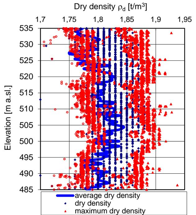
Fig. 11. Dry density values of the Czorsztyn Dam core material from control compaction tests.
