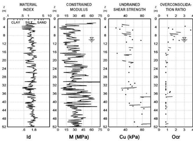
Fig. 9. Example of DMT results (performed after 10 years of exploitation of Czorsztyn Dam in the year of 2006).
