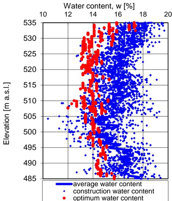
Fig. 10. Water content values of the Czorsztyn Dam core material from control compaction tests.
