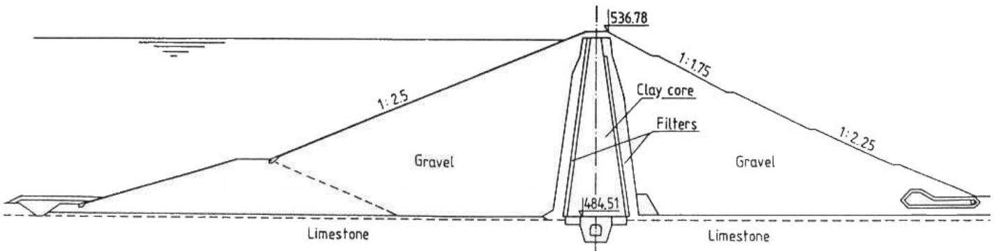
Fig. 1. Typical cross-section of Czorsztyn Dam.
