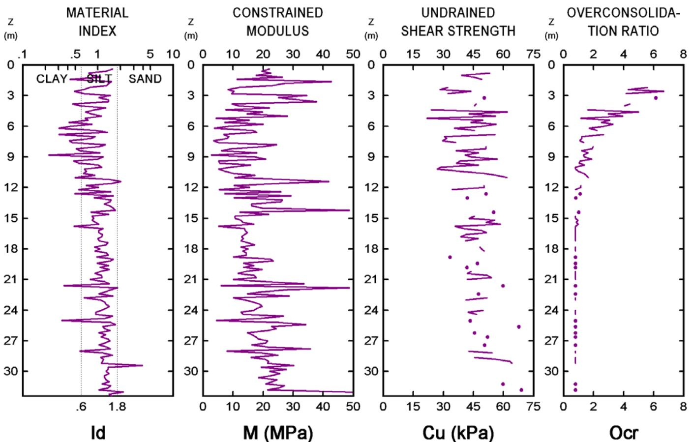
Fig. 4. Example of DMT result (performed from the 75 % of total core height of Świnna Poręba Dam)
