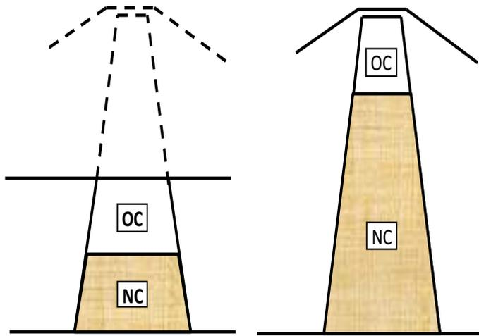
Fig. 14 The movement of prestressed (overconsolidated) OC and normally consolidated NC zones of the core during construction
