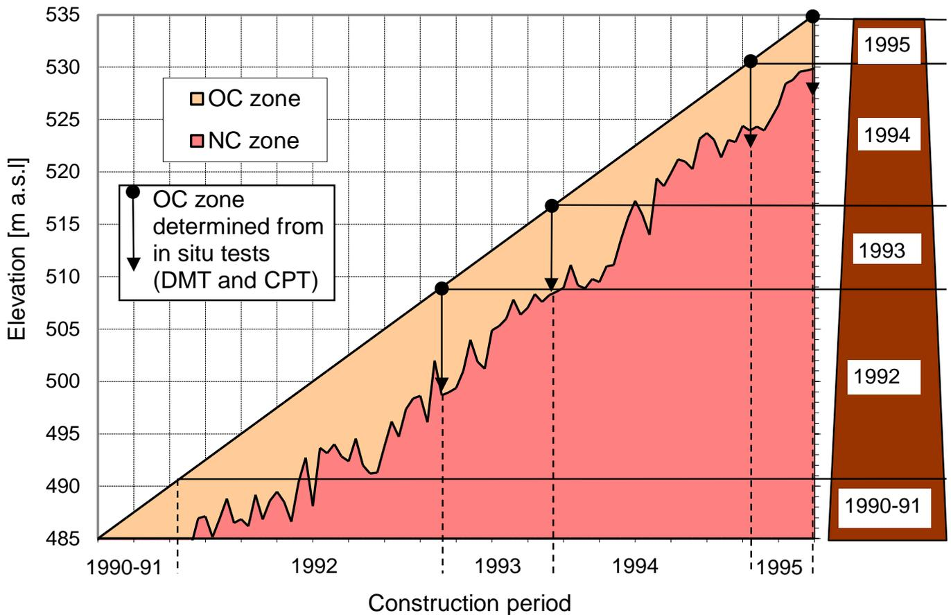
Fig. 13 Range of the overconsolidated OC zone of the core,  $\sigma_{ps}'$  calculated from the equation  $\sigma_{ps}' = 0.536e_o^{-7.83}$  and determined on the basis of CPT and DMT (Skutnik, 2002).
