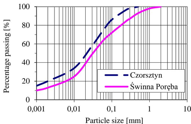
Fig. 3. Grain size distribution curves of the cores materials of Czorsztyn and Świnna Poręba Dams.
