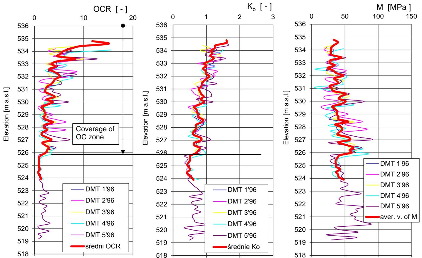
Fig. 8. Example of DMT results (performed at the end of construction of Czorsztyn Dam in the year of 1996).
